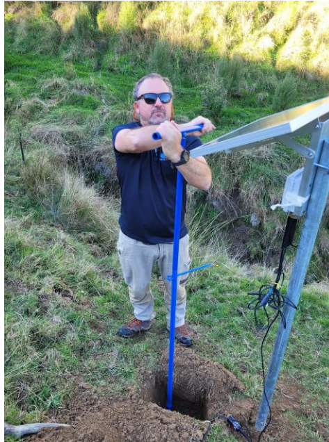
Figure A-1 Dr. Mick Aberton augering hole to install soil moisture probe 1
