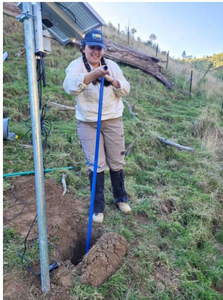
Figure A-2 Stephanie Phillips augering a hole to install soil moisture probe 2
