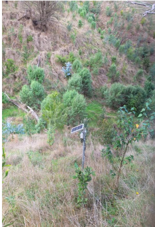
Figure A-8 Soil moisture probe 8 in revegetation area in colony (2 years post planting)
