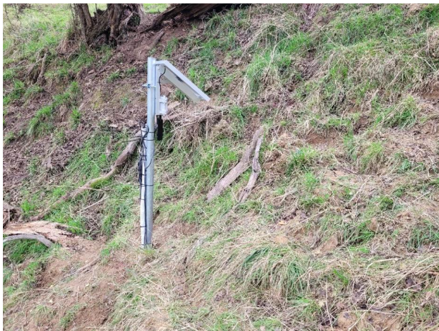
Figure A-5 Soil moisture probe 5, mid colony on steep slope
