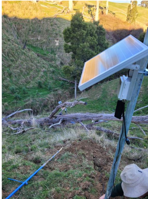
Figure A-3 Installation of soil moisture probe 3 with Solar array, datalogger and Wi-Fi aerial
