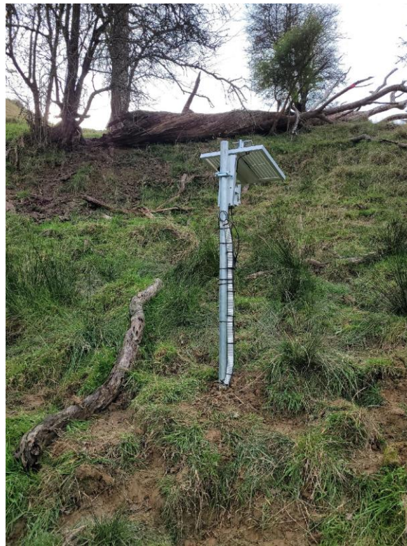
Figure A-6 Soil moisture probe 6, mid colony on steep slope
