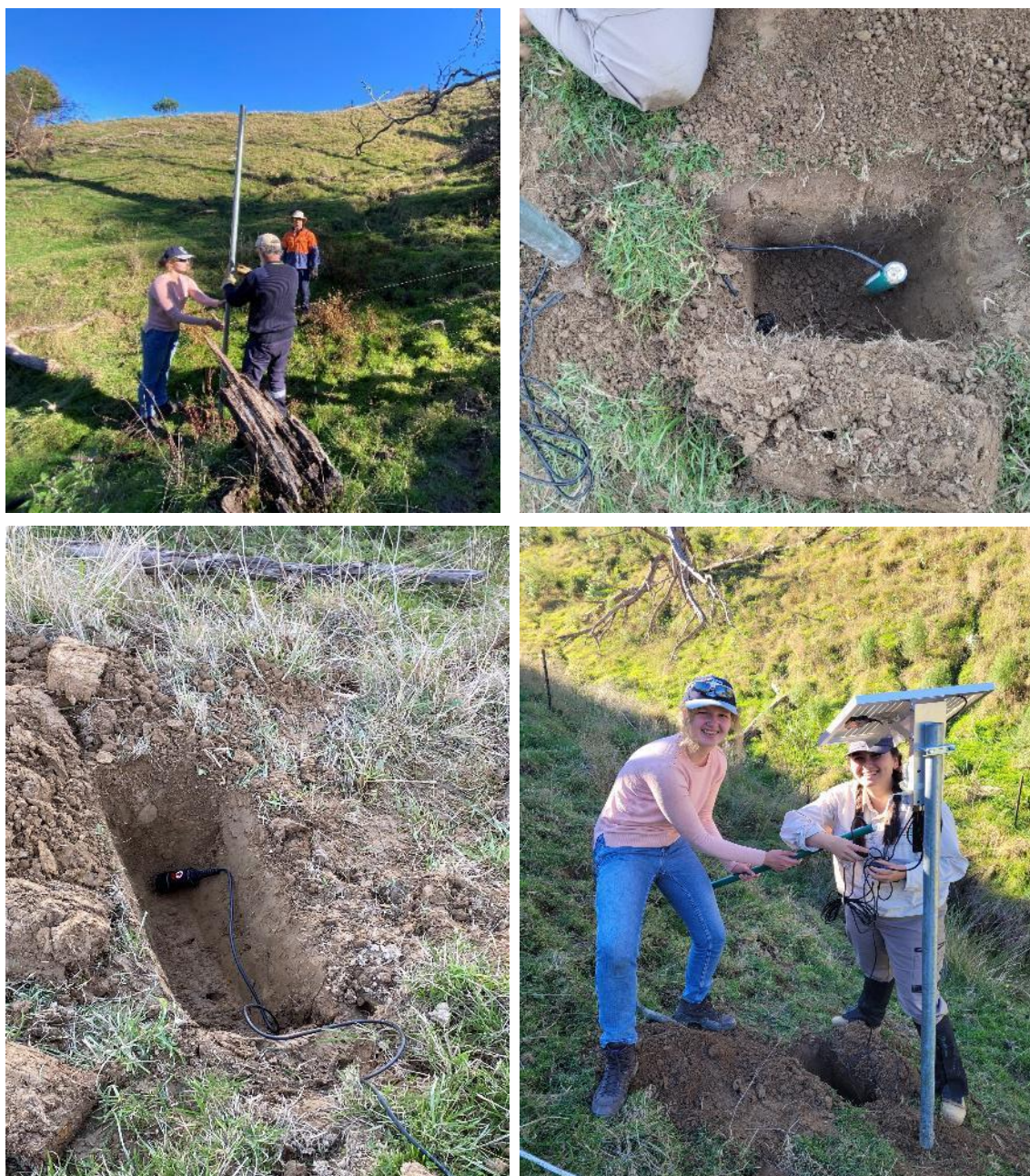
Photo 8 Installing hydrological monitoring probes at Site 1 Arawata
